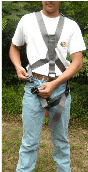
6. Connect the quick release buckles for each leg by inserting male end into female end you will hear it click it if is engaged. If you do not hear a click retry until you hear a loud click or do not use.
